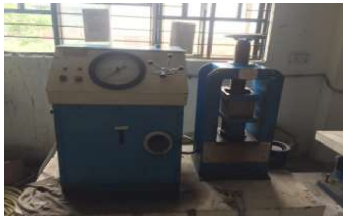
Fig.10 Experimental Setup for Compressive Strength Test
