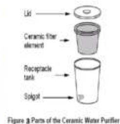
Figure 3 Parts of the Ceramic Water Purifier
