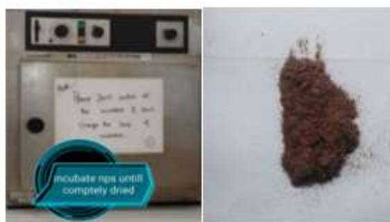
Figure 3.3 (a) Incubating sample until completely dried (b) dried sample
