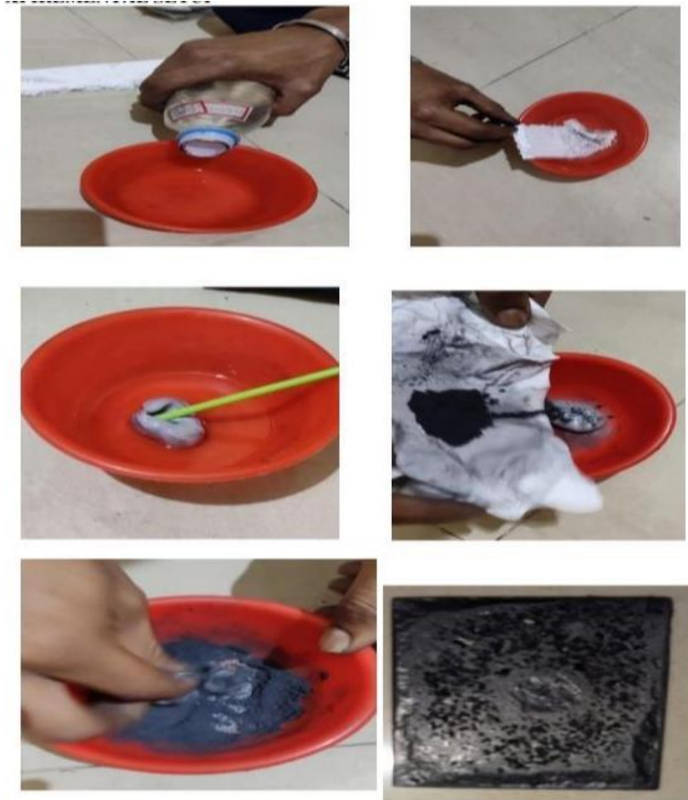
Fig1. Process stream outline portraying different stages for the amalgamation of GNs from squander plastics for TE applications.
