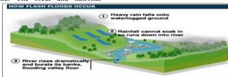
Figure 2: Flood occurrence mechanism(Source: Queensland development agency, 2012)
