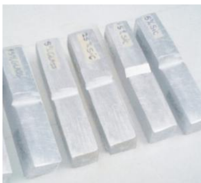
Figure 3.0: Impact Test Specimens Before Fracture (PTE Lab. FUTO, Owerri).
