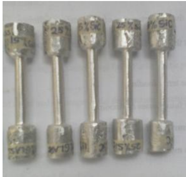
Figure 5.0: Tensile Test Specimens Before Fracture (Materials Lab. ESUT, Enugu).
