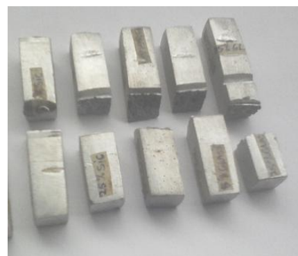
Figure 4.0: Impact Test Specimens After Fracture, (PTE Lab. FUTO, Owerri).
