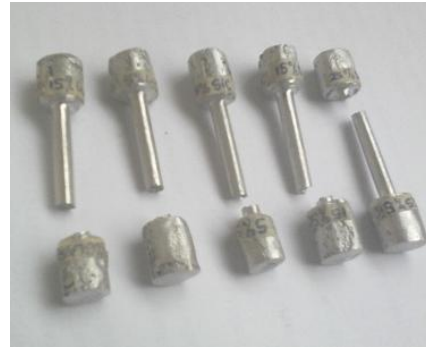
Figure 6.0: Tensile Test Specimens After Fracture, (Materials Lab., ESUT, Enugu).
