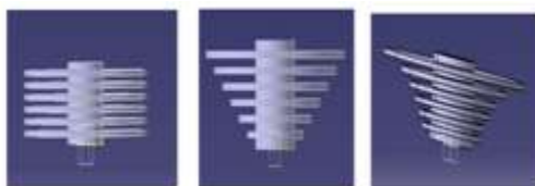
Fig-3 3D geometries of no varying fin, linearly varying fin, circular varying fin.
