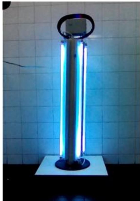
Fig. 6. UV-C device working. A video showing the setting up of the device is included in the supplementary material.
