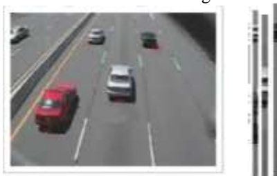
Fig 4: Current frame and extracted pixels on lane lines
