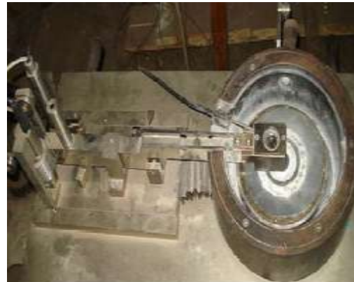
Fig.1: Pin on Disk Tribometer
