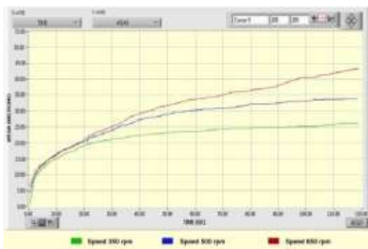
Fig.6: Effect of Sliding Speed on Wear
