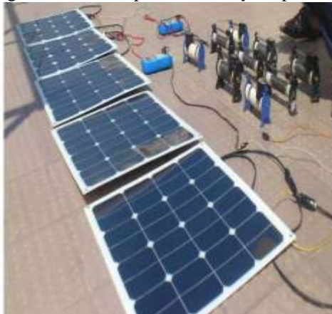
Fig. 3.3 solar (PV) panel used in operation of EV
