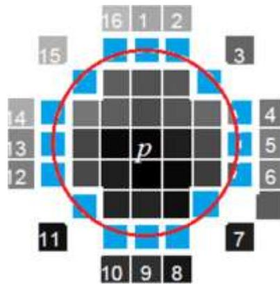
Fig 2: FAST detector
