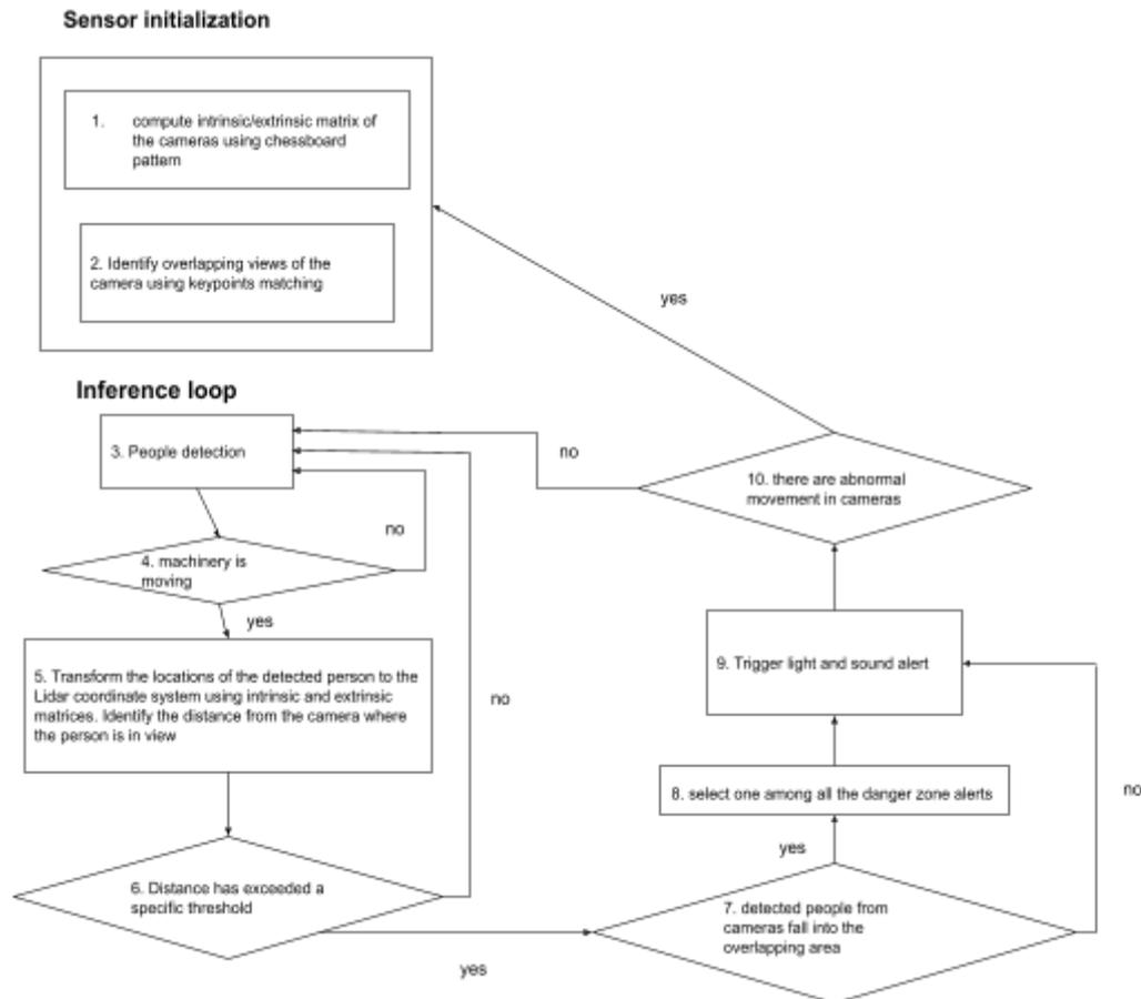
Fig 2: System Architecture of DZASS
