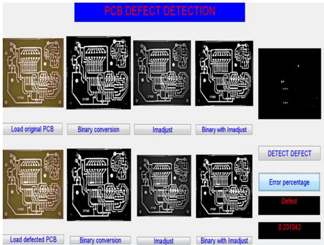
Fig 7. GUI showing error percentage in PCB
