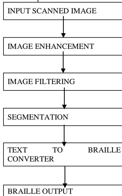
**Figure 4. Functional Diagram of Braille**
