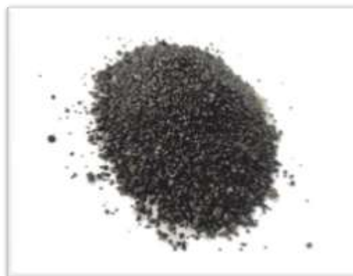
Figure 1.1 – Copper Slag sample
