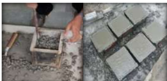
Figure 3.2- Casting of cubes
