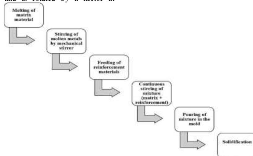
**Fig.1 Fabrication Flow Chart**
