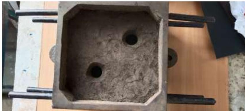
**Figure 3:** MOLD CAVITY
