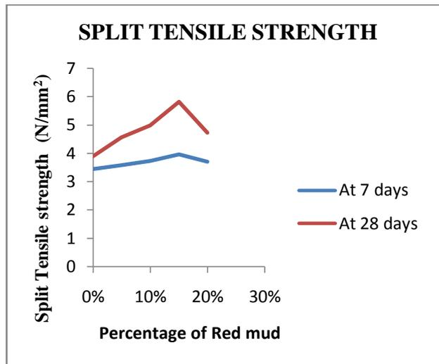
**Fig 4.2 Split Tensile strength Result**
