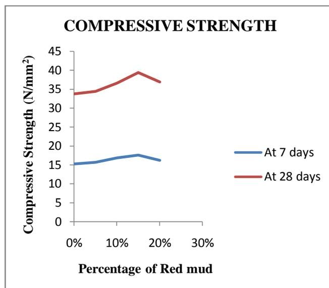
Fig 4.1 Compressive strength Result
