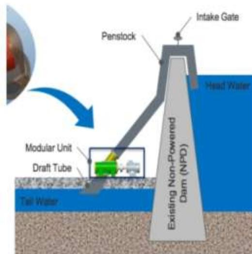
Fig. 3: Powering of Non Powered Dams
