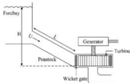
Fig. 1: A Small Hydropower Plant
