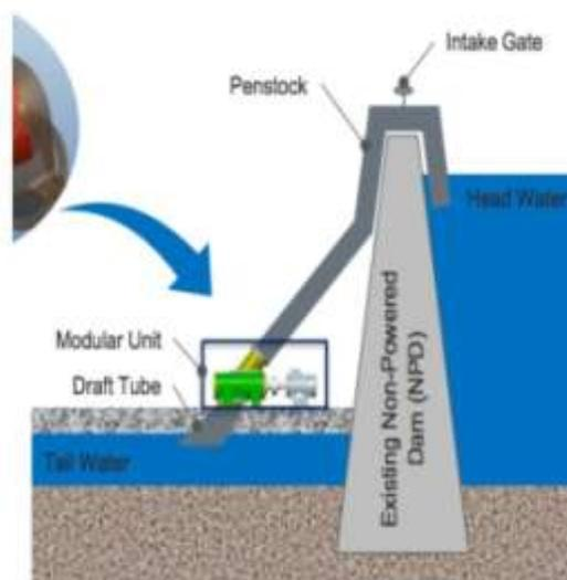
Fig. 3: Powering of Non Powered Dams
