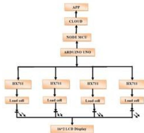
Figure 1:Block Diagram of Proposed Model
