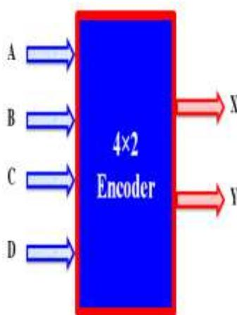
Fig.1 Block diagram of 4x2 encoder
