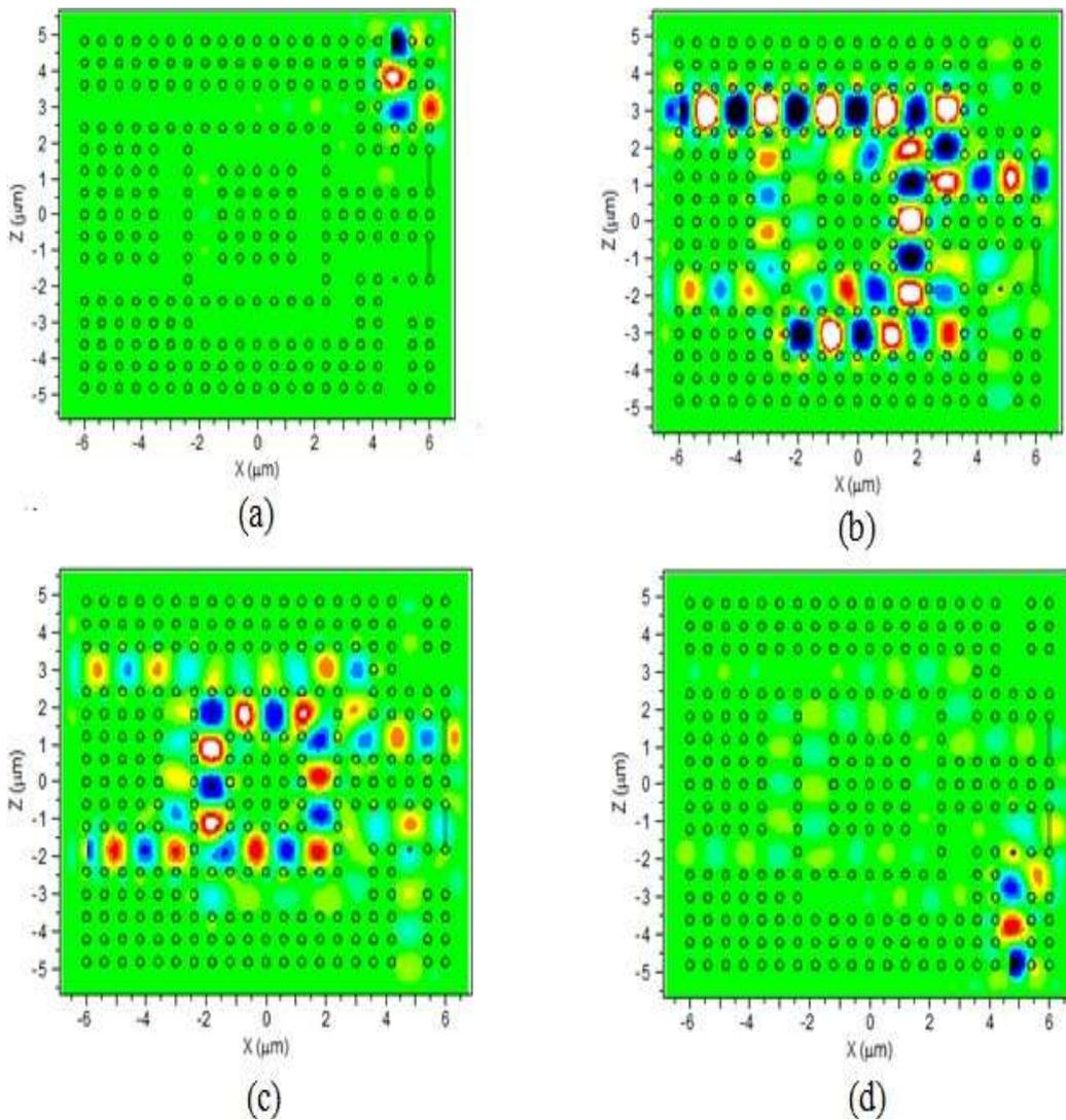
**Figure .3 Steady-state distribution for the input pattern a ABCD=1000, b ABCD=0100, c ABCD=0010, d ABCD=0001.**
