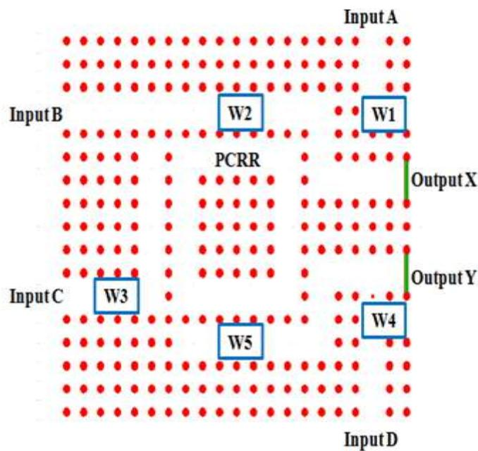
Figure .2 The structure of layout with optical encode
