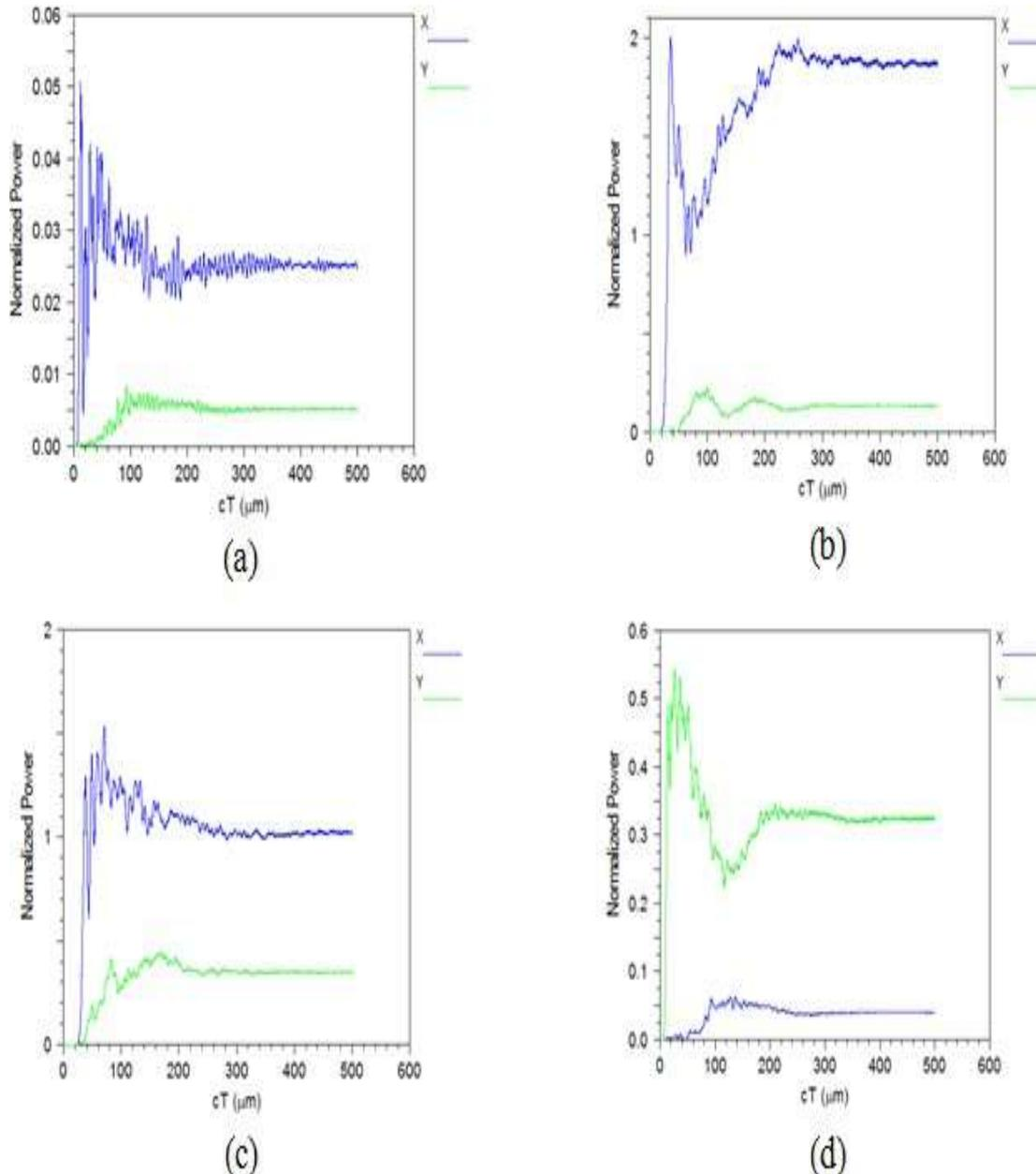
**Figure 4** The time response of the normalized output power for a ABCD=1000, b ABCD=0100, c ABCD=0010, d ABCD=0001
