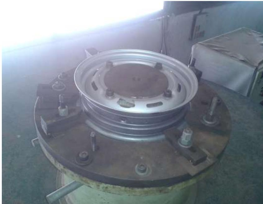
**Fig.2. Photograph Cornering Fatigue Test Rig.**
