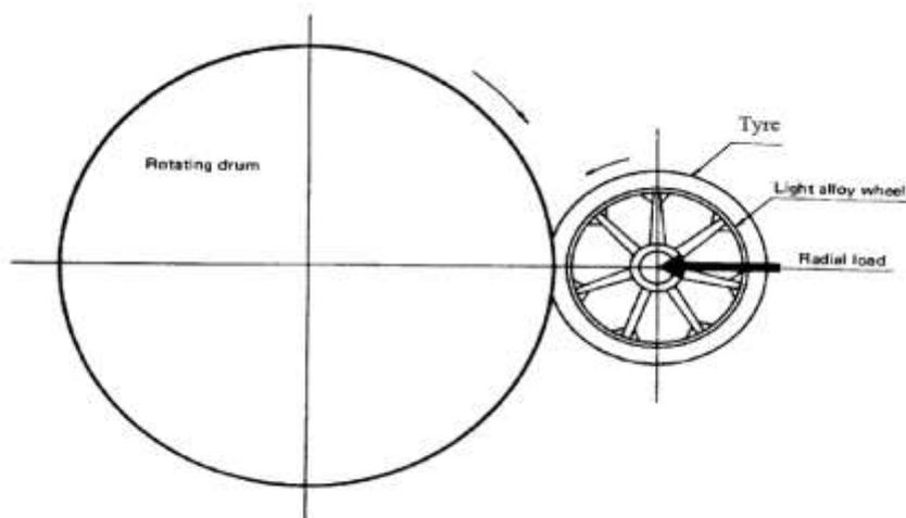
**Fig.3 General view of the wheel dynamic radial fatigue test.**
