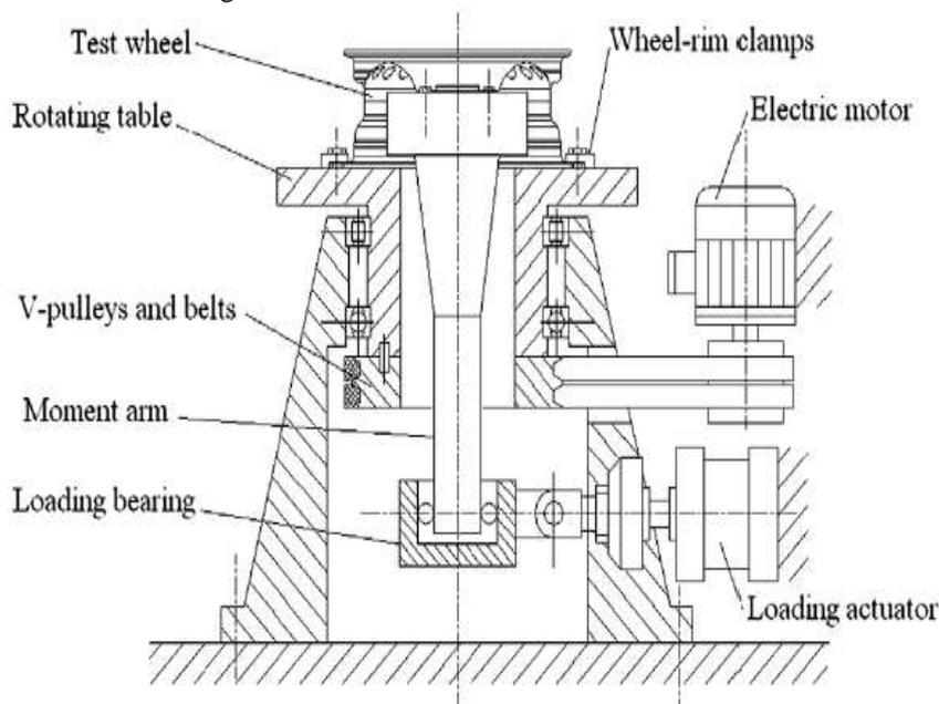
**Fig 1.Schematic of Cornering Fatigue Test Rig.**
