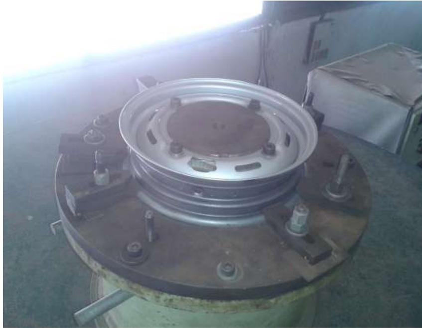
**Fig.2. Photograph Cornering Fatigue Test Rig.**
