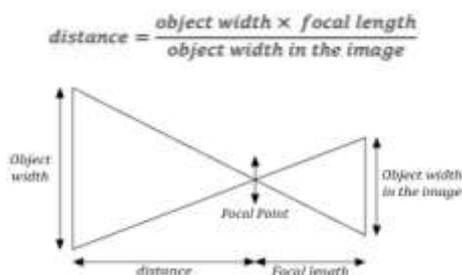
Figure 2 Calculating distance from image
