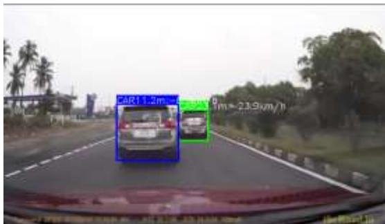
Above diagrams shows the result of the proposed algorithm. In those images the objects are represented with boxes and the class of the object along with distance and speed is displayed above the object.
