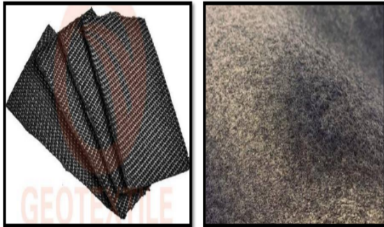
(a) Woven Geotextile (b) Nonwoven Geotextile Fig.1.Geotextile
