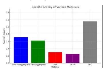
The bar chart illustrates the specific gravity of five different construction materials, highlighting OPC (Ordinary Portland Cement) as having the highest specific gravity at 3.15, indicating it is the densest of the materials shown. Coarse Aggregate follows with a specific gravity of 2.72, then Fine Aggregate at 2.62, demonstrating slightly less density. The lightest materials are SNA (Super Naphthalene Aluminate) and GCHA (Ground Hydrated Aluminate) with specific gravities of 2.30
