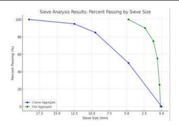
For the coarse aggregate, represented by the blue line, the curve starts at 100% passing and gradually declines as the sieve size decreases, showing a more gradual retention of particles across the range of sieve sizes until reaching 0% passing at the smallest size (0 mm).
