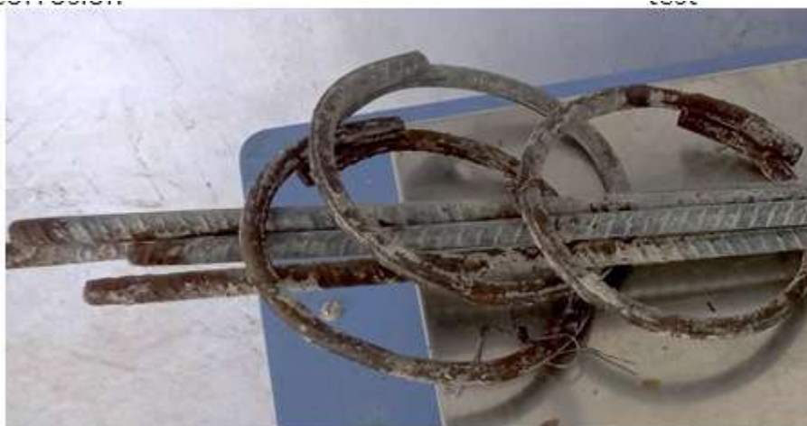
Figure6:View of reinforcements after accelerated corrosion test
