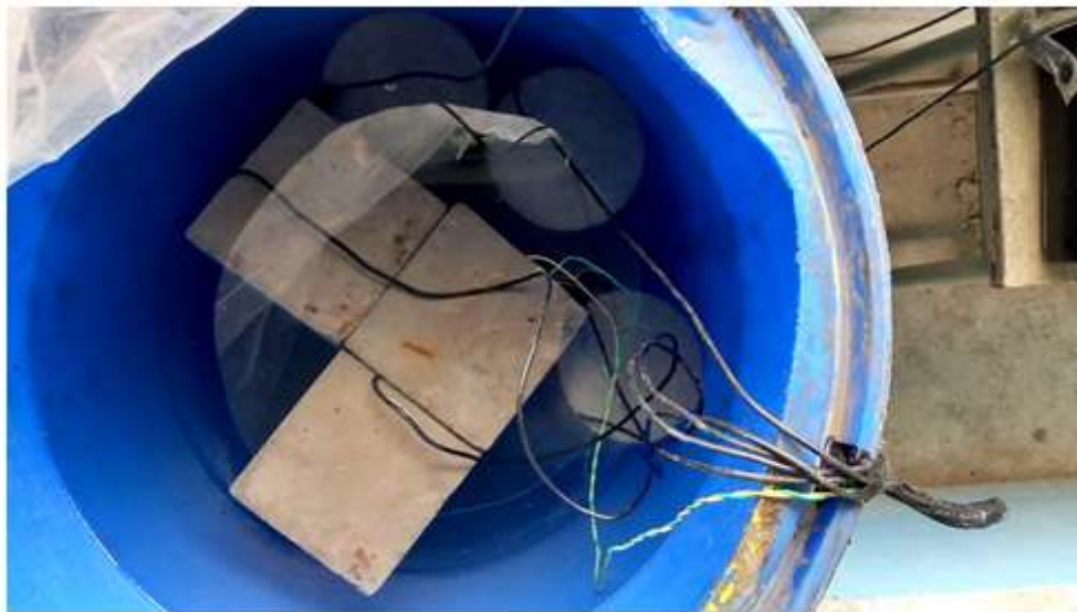
Figure 4 : Specimens under water tank with 0.5 % NaCl Solution
