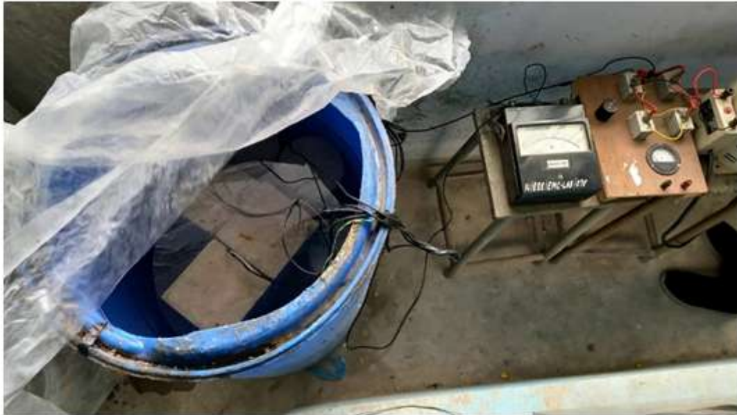
Figure 3 : View of Accelerated Corrosion Technique
