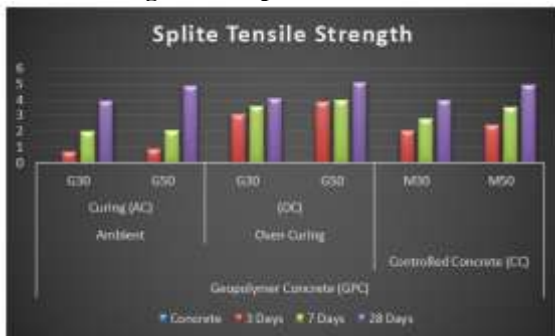
Figure 4.4: Split Tensile Strength (MPa) of Geopolymer concrete
