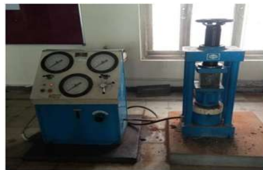
Figure 4.2: Compressive Strength Testing Machine
