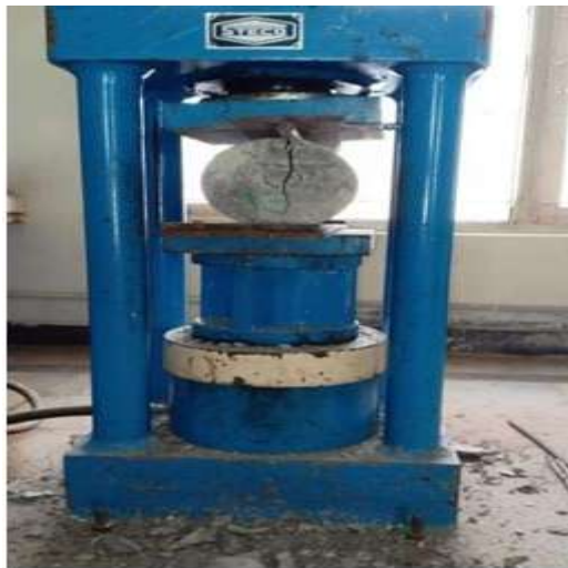
Figure 4.3: Split Tensile Test
