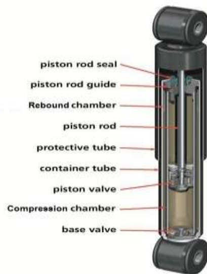
Fig.1 Twin Tube Shock Absorber
