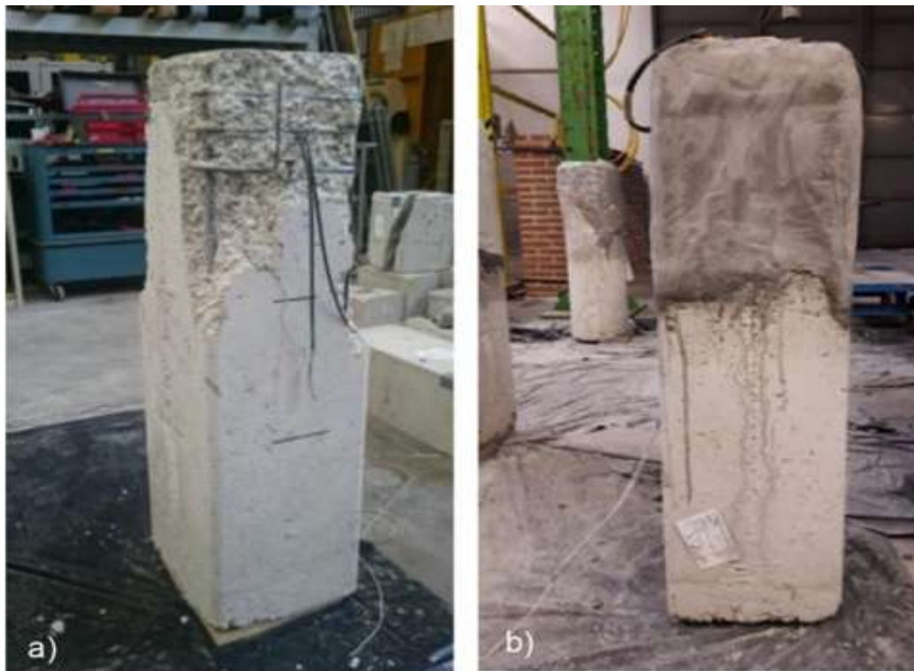
Fig. 3. S33_NC specimen after failure (a); S33_NC specimen after repair operation ( b ).
