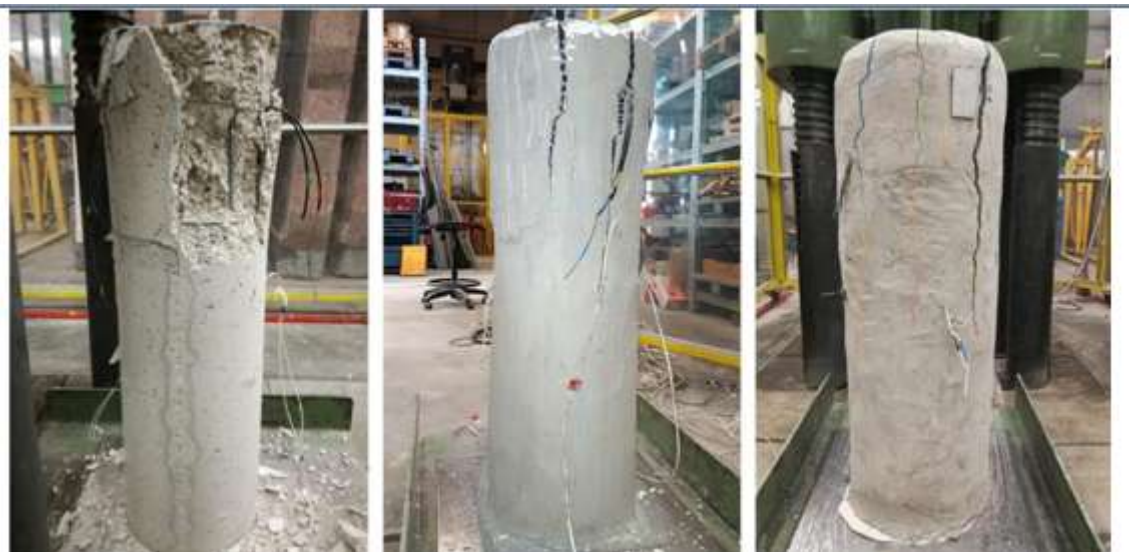
Fig. 5. C20_NC, C20_D0_C2 and C20_D1_C2 at the end of the loading history.
