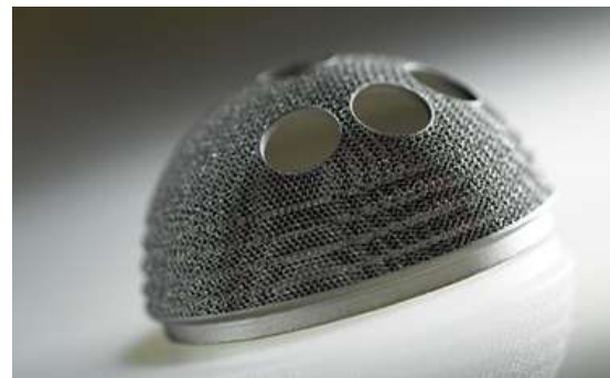
5.3. A titanium hip cup created with additive manufacturing
