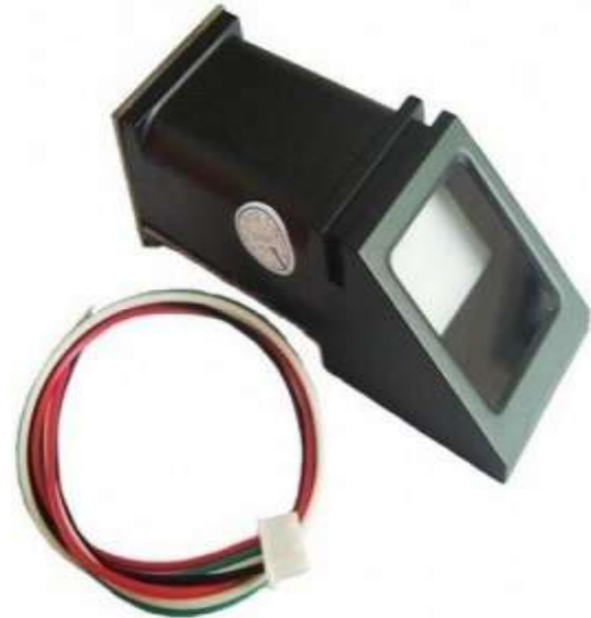
Fig 3.6: Fingerprint module (FPM10A)
