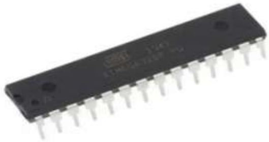
Fig 3.5: Diagram of the ATmega328p Microcontroller
