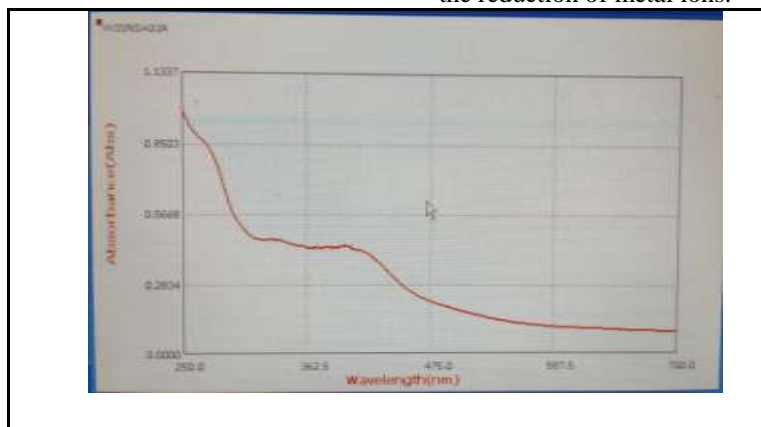
Fig. 3: UV-Vis spectra of AgNP using cross-linked wheat extract and sodium alginate
