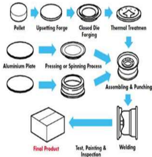
Figure 16: Forging method (three piece rim)
