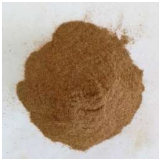
Plate 2: Alkaline Treated Groundnut Particulate
