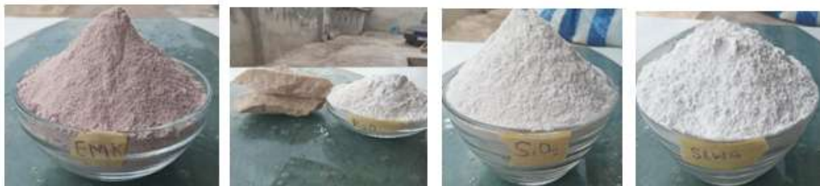
Ehime Mbanjo -EMK Feldspar- AFJ Silica- IJS SLWG- Waste glass Plate 1. Processed Raw Materials
