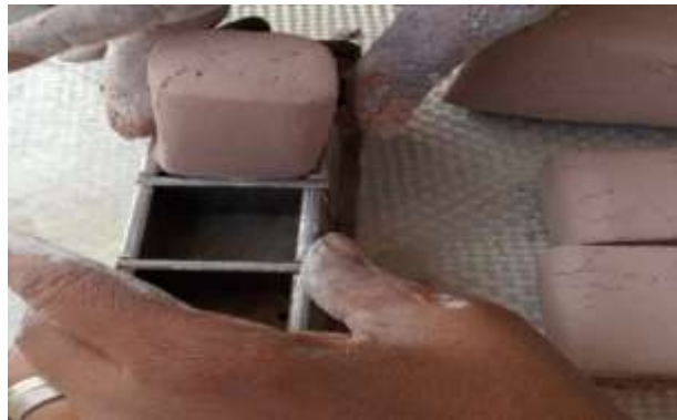
Plate 2: Making of Samples with 40×40mm Iron Mould
