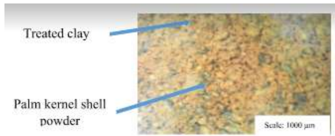
Fig 18: mixture of 70% treated clay and 30% palm kernel powder seen with a USB digital microscope.
