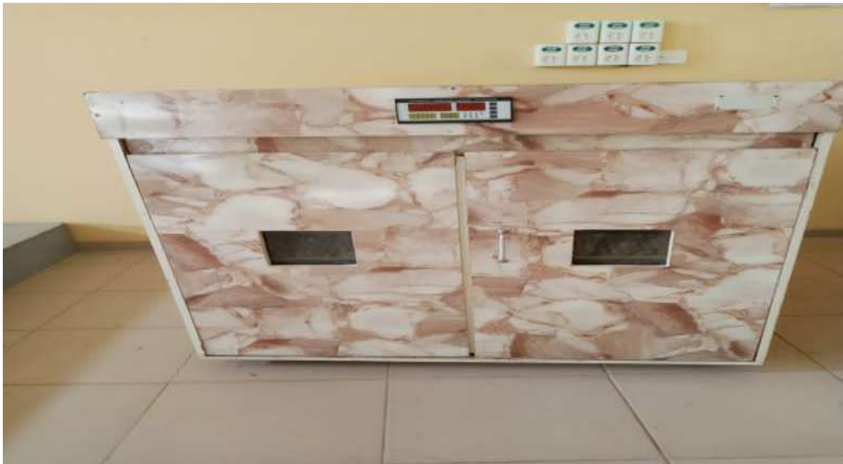
Plate 4.1: Egg Incubator with MDF Plywood.
