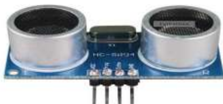
Fig. 6: Ultrasonic Sensor for Obstacle Detection.
