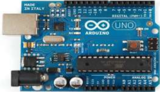
Fig. 2: Arduino Uno Development Board with ATmega328p Microcontroller.
