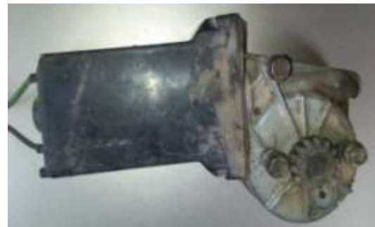
Fig.4: D.C Motor for Wheelchair Drive.
