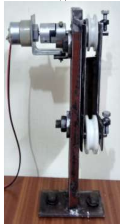
(c) Figure 12 (a) Front View (b) Side View (c) Fabricated Idler Setup and Adjustable Holder
