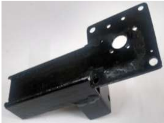
(c) Figure 11 (a) Front View (b) Side View (c) The Fabricated Winder Motor Housing
