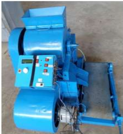
Fig. 3: Fabricated Automated shelling Machine
