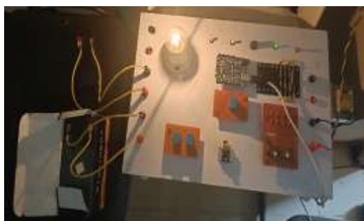
FIG 5: Hardware of EV battery charging by multiple sources
