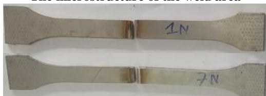
Image of welded sample after tensile test The average tensile strength results of the samples
