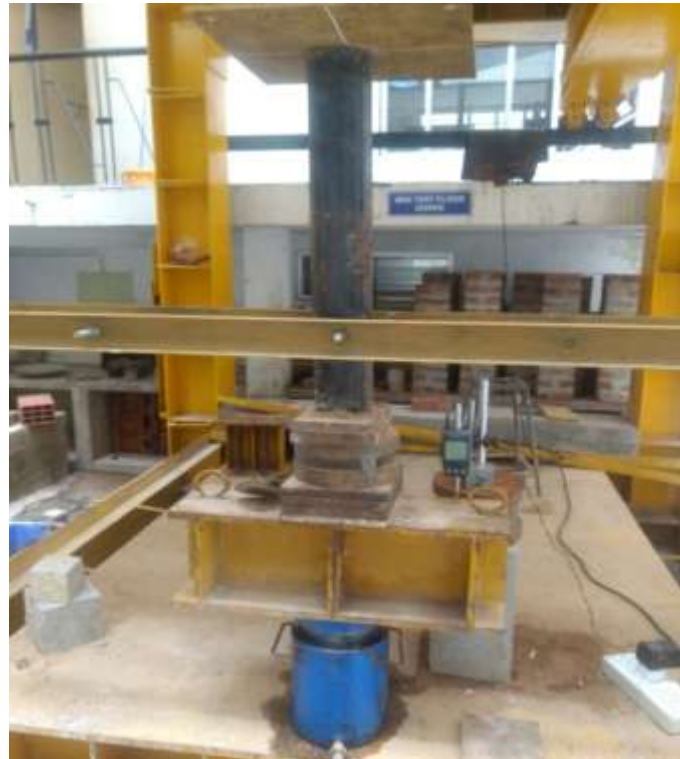
FIG-3: Experimental setup for axial-compressive loading
