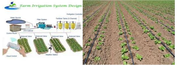
The diagram illustrates a modern Farm Irrigation System Design that integrates automation and smart technologies to improve irrigation efficiency. The process begins with a water source, from which water is drawn and passed through a filter system to remove impurities. This is a smart irrigation system that uses cloud control, sensors, and automated valves to deliver precise amounts of water and fertilizer to different sections of farmland.
