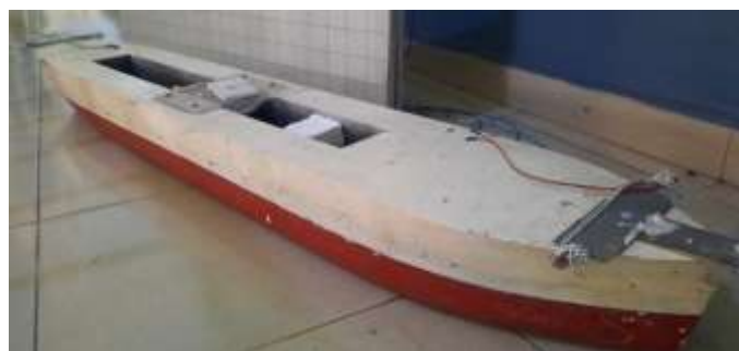
Figure 3: Mystery FPSO Wooden Experimental Model.
