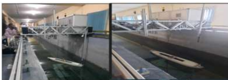
(a) Wooden FPSO Model at Oblique sea condition during experimental studies
