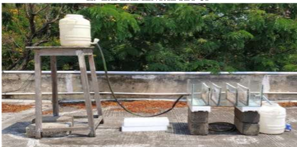
Figure 1 Photographic View of Artificially Constructed Wetland Setup
