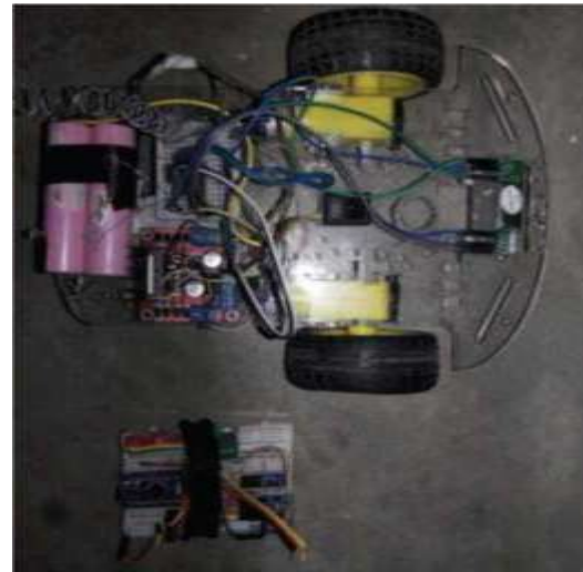
Fig. 4. Designed prototype with transmitter, receiver and robot.
