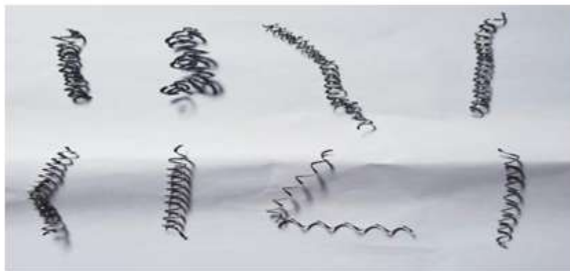
Fig 1 Chips formed during machining (TiN Coated tool)
