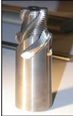
Fig.1.7:- A solid multiple-form thread milling cutter.
