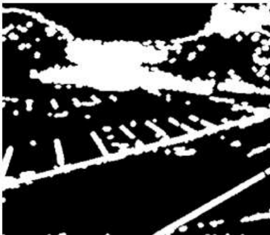
Fig. 8. Dilated edge image with holes filled
