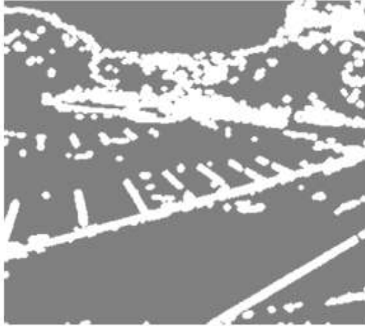
Fig. 7. Resulting edge image after fourth dilation
