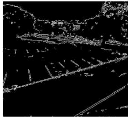
Fig. 6. Strong edges identified in binarized test image using the Canny edge detection algorithm.
